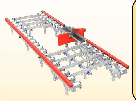
Thin Kerf sawing will yield up to 30% more yield over circle sawing, the Go Fast Go-Around Grade System is a heavy duty, high capacity, and economical solution for your grade sawing operation. This system comes complete: heavy duty built low profile saw, outfeed rolls with cant tipper, heavy duty cross over chains, infeed chains with turn, variable feed speed, quick adjust blade tracking and much more.
